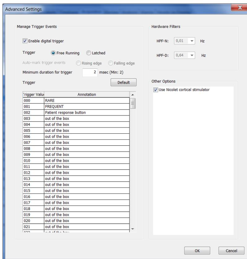
In Free Running mode, every change on the 8 inputs generates an event in the NeuroWorks study. This mode is typically used when trigger pulses arrive at different timing on each of the 8 input ports. Resulting in the following trigger values:
