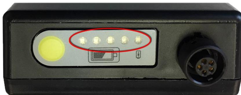
Provided that the internal temperature of the breakout is not too high, the internal battery is automatically recharged when the external battery is connected or when the breakout is reconnected to the Base unit.
