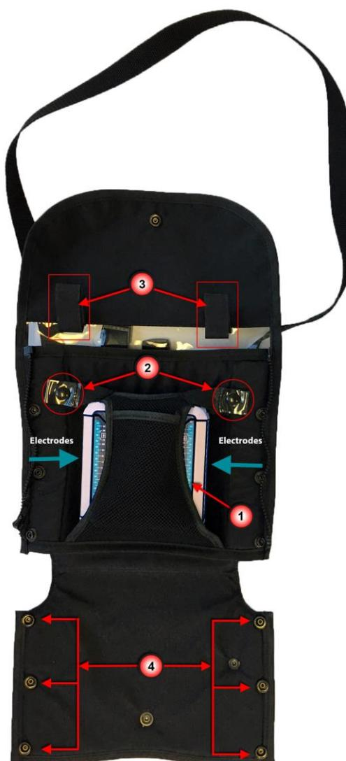
4. The wired connections, such as the breakout to breakout or breakout to Main cable(s), and secured through the loops provided. The pouch should then be closed by snapping the outside snaps together to enclose the breakout box(es) completely.
