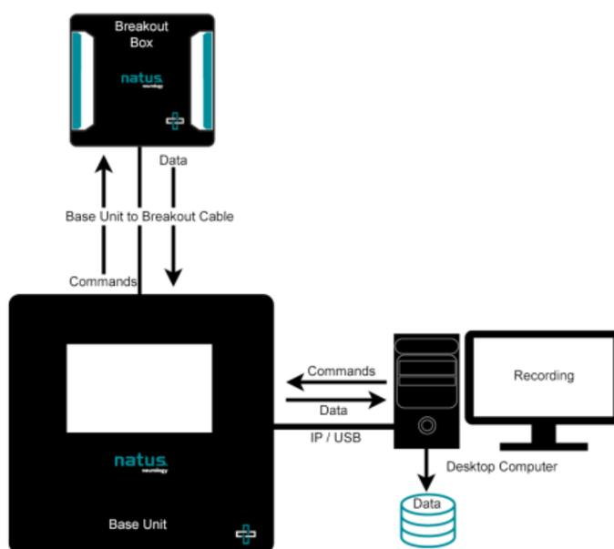
Figure 1: Physical Connection of the Quantum System
