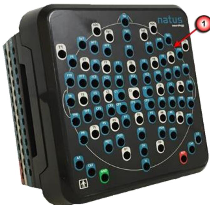
1 Standard 10-10/10-20 Channel Inputs. See [Connecting the 10-10/10-20 Pin box to the Quantum Breakout](#) for additional information.
