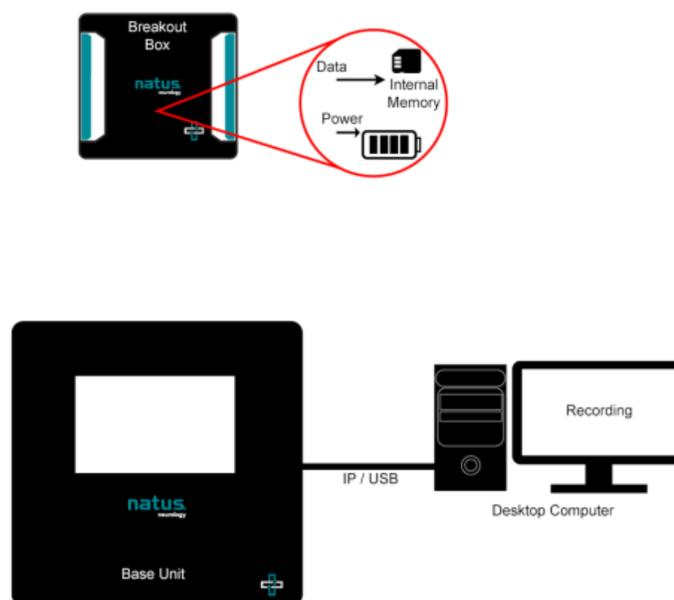
Figure 2: Physical Disconnection of the Quantum System – Ambulatory Mode
